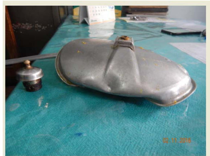
Figure 3: Photograph showing the buckled lid of the cooker.
