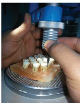
Figure 3: cavities realization using a milling machine (F4 basic, DEGUDENT)
