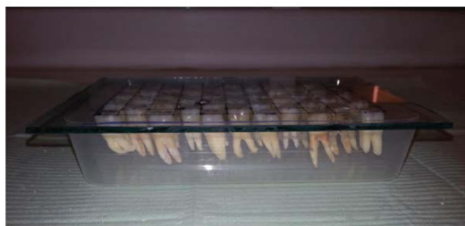
Figure 1: sixty teeth bonded by their occlusal surfaces on a glass plate
