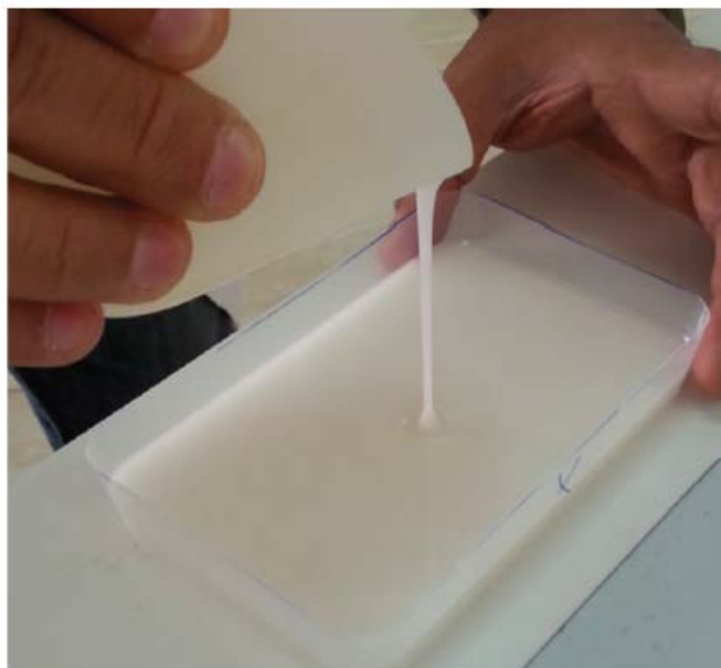
Figure 2: preparation of the resin material before the inclusion of the teeth in it
