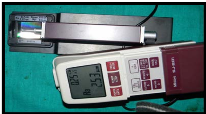
Figure 6: Surface Profilometer (Mitutoyo – SJ-201, Mitutoyo Corp, Kawasaki, Kanagawa, Japan)
