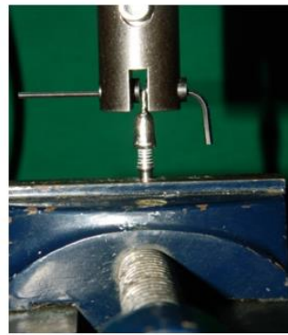
Figure 7: Removal of coping from abutment after pull out test
