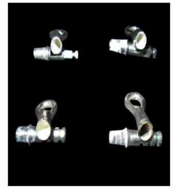
Figure 8: Copings and Abutments showing cement failure mode
