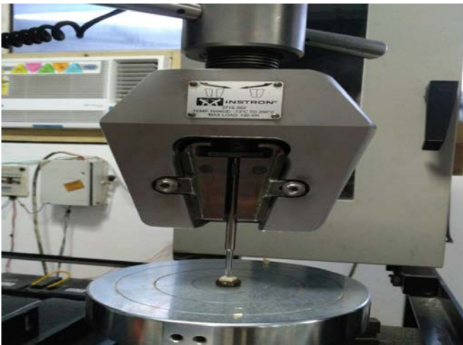
Figure 1: Testing of flexural strength by Universal Testing Machine
