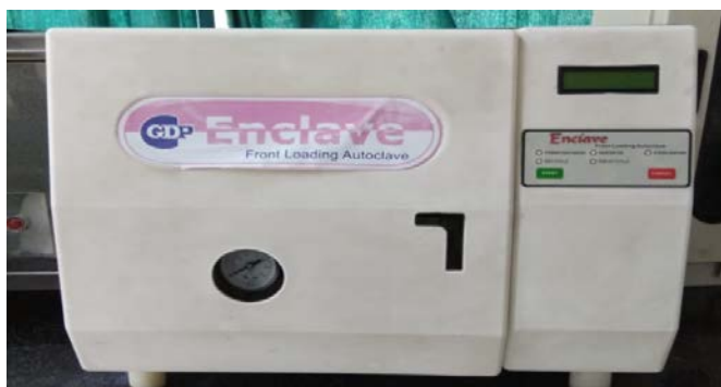
Fig 7: front loading autoclave
