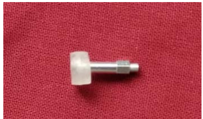
Fig 6: customized connector to attach smart peg with mini implants
